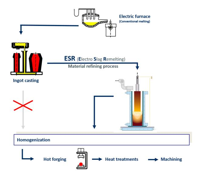
"The ESR remelting process is recognized as the cutting-edge production process for the production of high-performance materials that must withstand high stresses"
