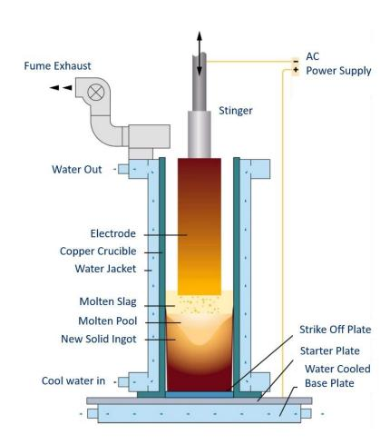
The steel block obtained by this ESR remelting / refining is very homogeneous and of a high degree of sulfidic and oxidic purity.
